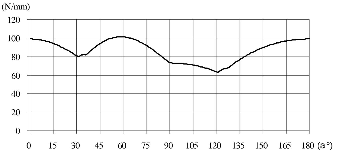
**Figure A3.** Characteristic plate capacity for shear  $f_{v,a,k}$ .
