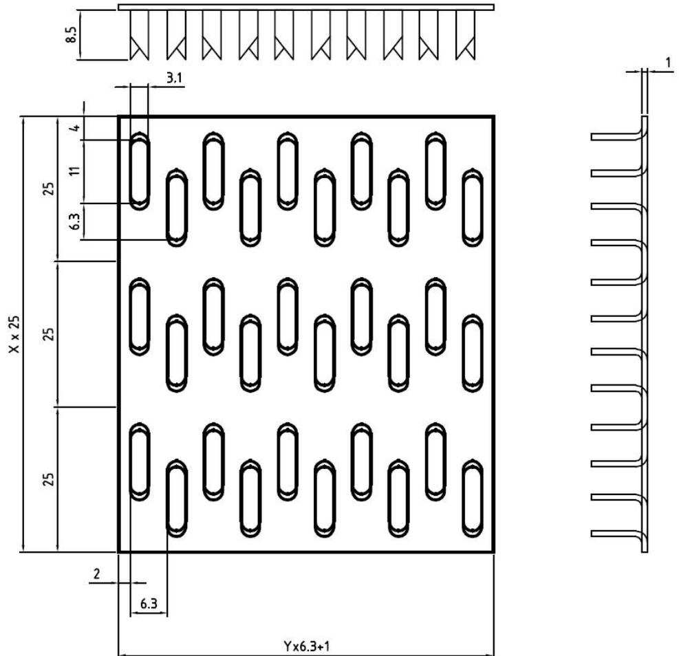
Figure 1. Structure of LL10 nail plate.
