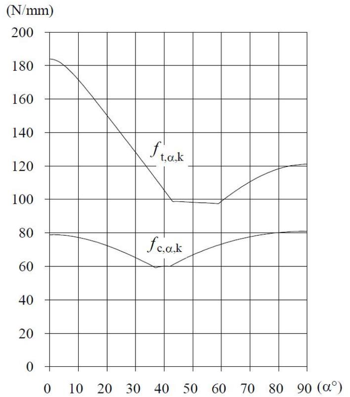
**Figure A2.** Characteristic plate capacities for tension ( $f_{t,\alpha,k}$ ) and for compression ( $f_{c,\alpha,k}$ ).
