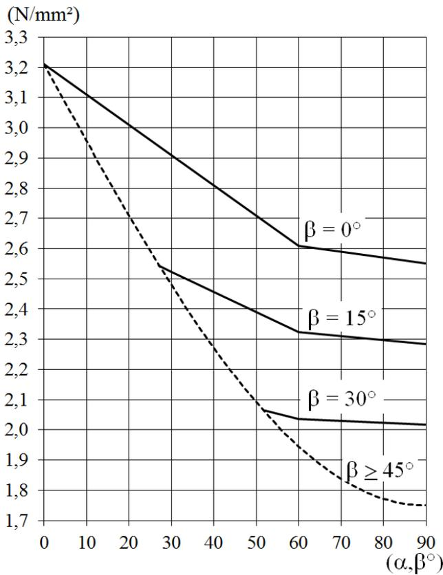
**Figure A1.** Characteristic anchorage strength  $f_{a,a,b,k}$  for solid timber in strength class C24. The minimum curve (dash line) is used for direction angle  $\max(a,b)$ .
