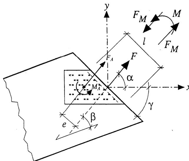
Figure 2. Geometry of nail plate connection loaded by a force  $F$  and moment  $M$ .
